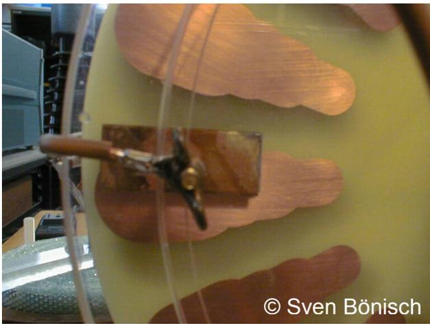
Fig. 6: Electrode setup from the side
