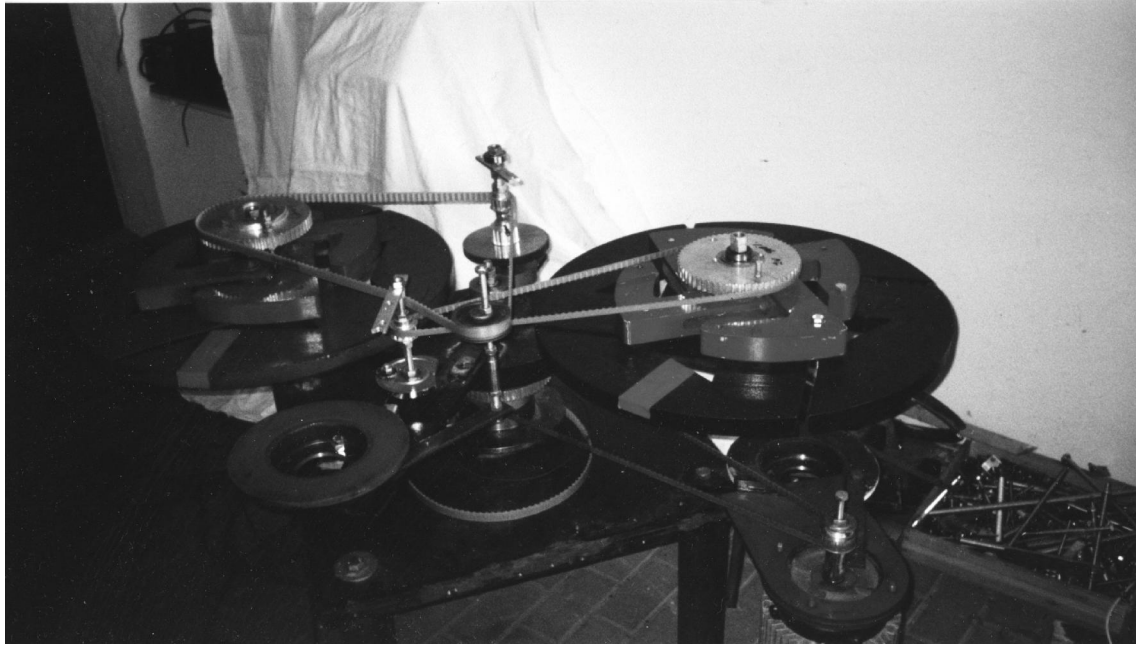
Fig.3: Wuerth's setup of the parametric rotator During our measurements the belts were completely removed. The same holds for the red swastikas and the red parts inserted in the big disks.
